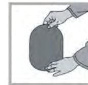
1. Apply the self-adhesive template to the duct wall (included with the product). The prices shown do not include VAT or transport
