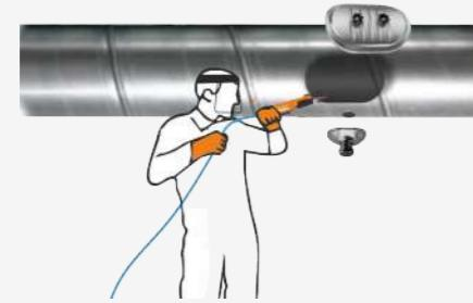
Drains made of stainless steel for the evacuation of chemical or other liquids during duct cleaning. Corrosion resistant and totally watertight material.
